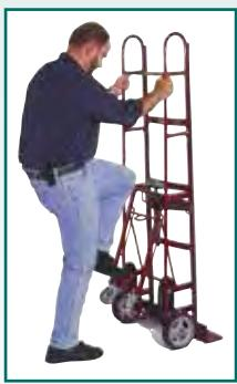
Improved kick-out design allows operator to kick-out wheels with both hands on the truck.
