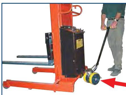
5th Wheel Steering Option for easier mobility and precision steering in confined areas. Available only on 1,500 and 2,000 lb models. 8" locking polyurethane wheels. Spring loaded handle. Turning radius: 73.5". Can be field installed. Order as separate option under Part # 261099
